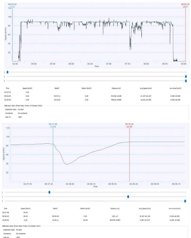
Above, Tachograph data from the HGV, assessing speed and driver behaviour
