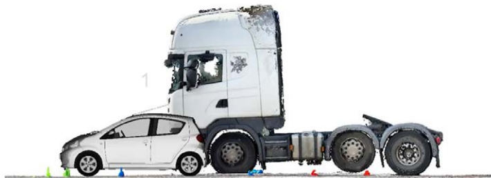
Above, 3D digital model to show the position of the vehicles at the time of the collision
