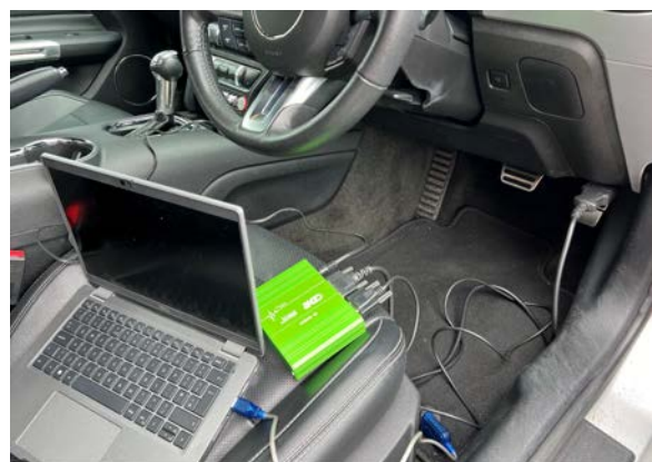
Figure 1: EDR download being conducted on the vehicle, with the recovery equipment connected directly to the vehicle's OBD port.
