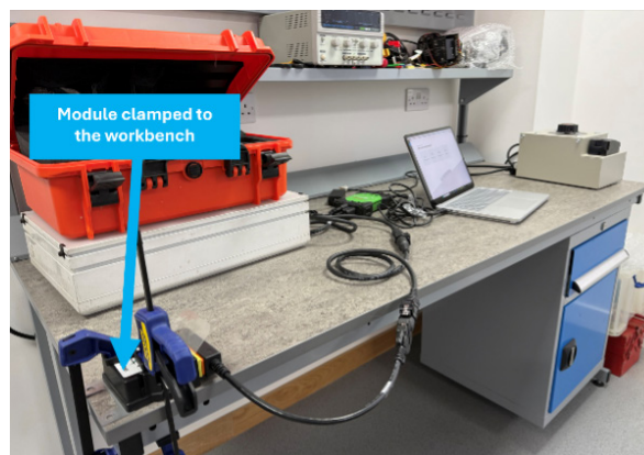
Figure 2: EDR data being recovered directly from the module at Hawkins forensic lab in Manchester.
